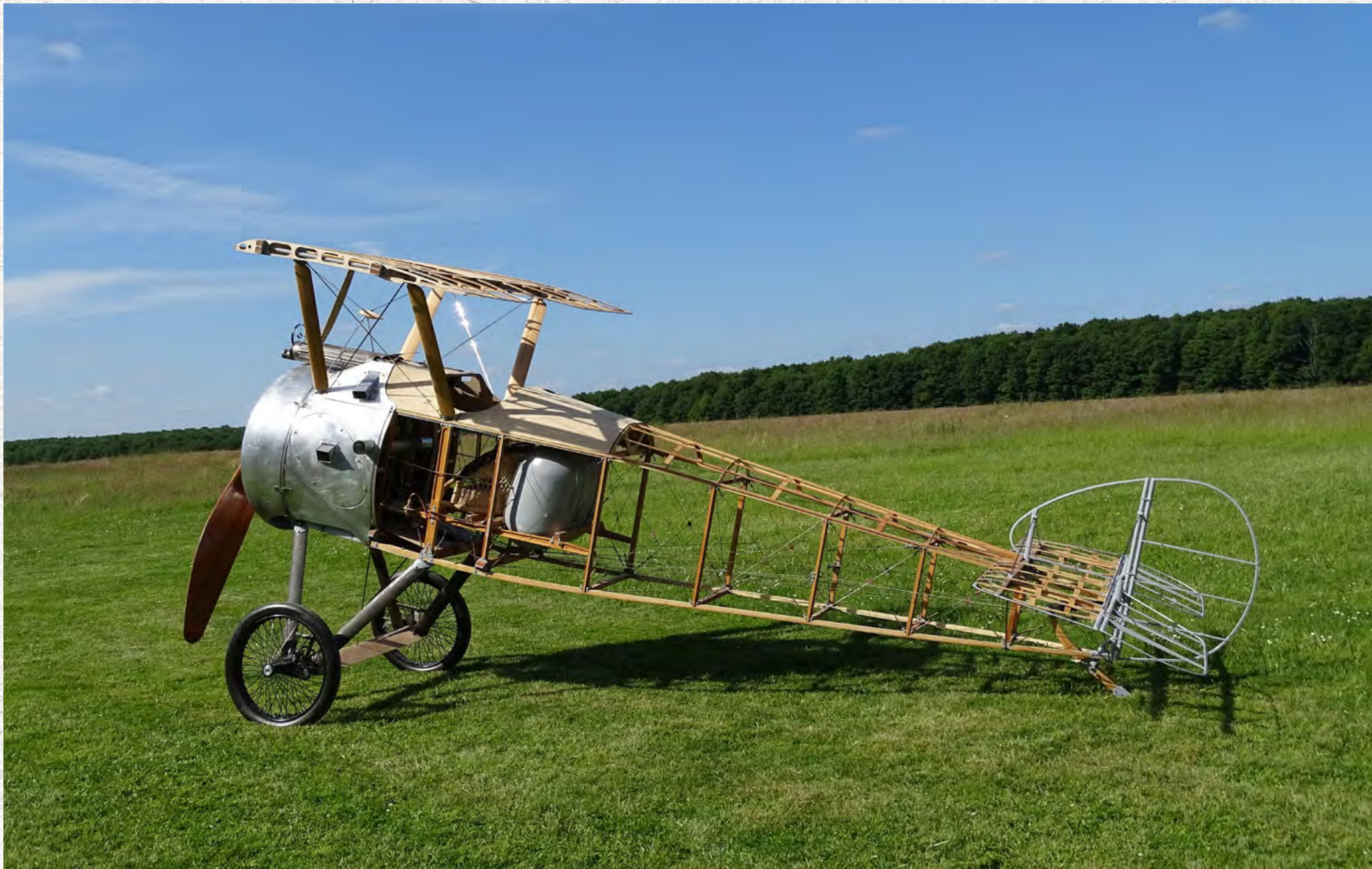
A replica of a First World War Sopwith Camel aeroplane, with a basketwork seat visible in the cockpit. To save weight, aircraft had openwork wooden frames with linen stretched over them. Courtesy of John S. Shaw.
