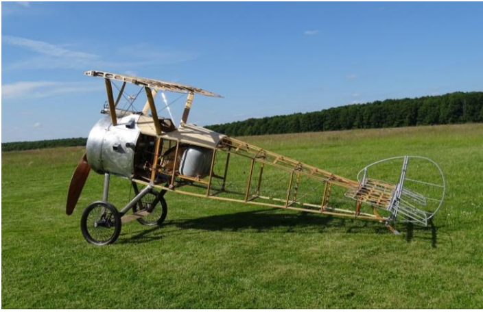
Image: A replica of a First World War Sopwith Camel aeroplane built by John Shaw, with a basketwork seat visible in the cockpit. To save weight, aircraft had openwork wooden frames with linen stretched over them. Courtesy of John S. Shaw.
